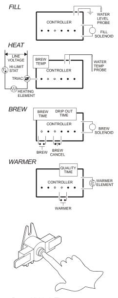
Reset Hi-Limit Thermostat 240 V & Dual Voltage Units
